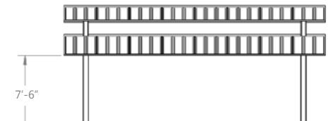
Minimum Clearance Height w/ MR Roof
