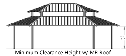
Minimum Clearance Height w/ MR Roof
